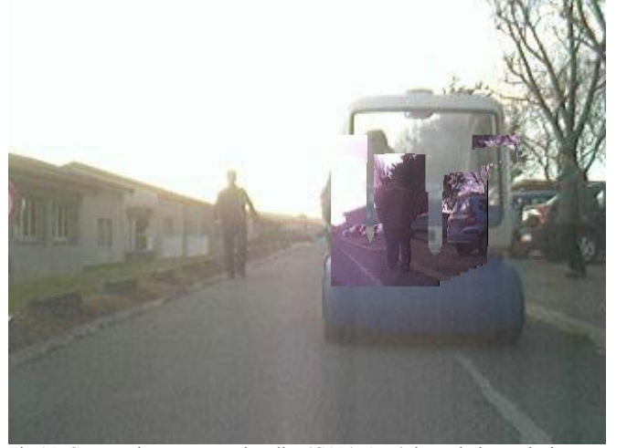
Fig.15. Cooperative augmented reality (CAR): ‘see’ through the occlusion
