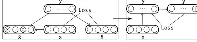
**Fig. 5** The training scheme of an SDAA. Input components modified by the corruption process are marked with a  $\otimes$  cross and code components modified by the sparsification process are marked with a  $\oplus$  cross.
