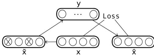
**Fig. 3** The training scheme of a DAA. Input components modified by the corruption process are marked with a  $\otimes$  cross.
