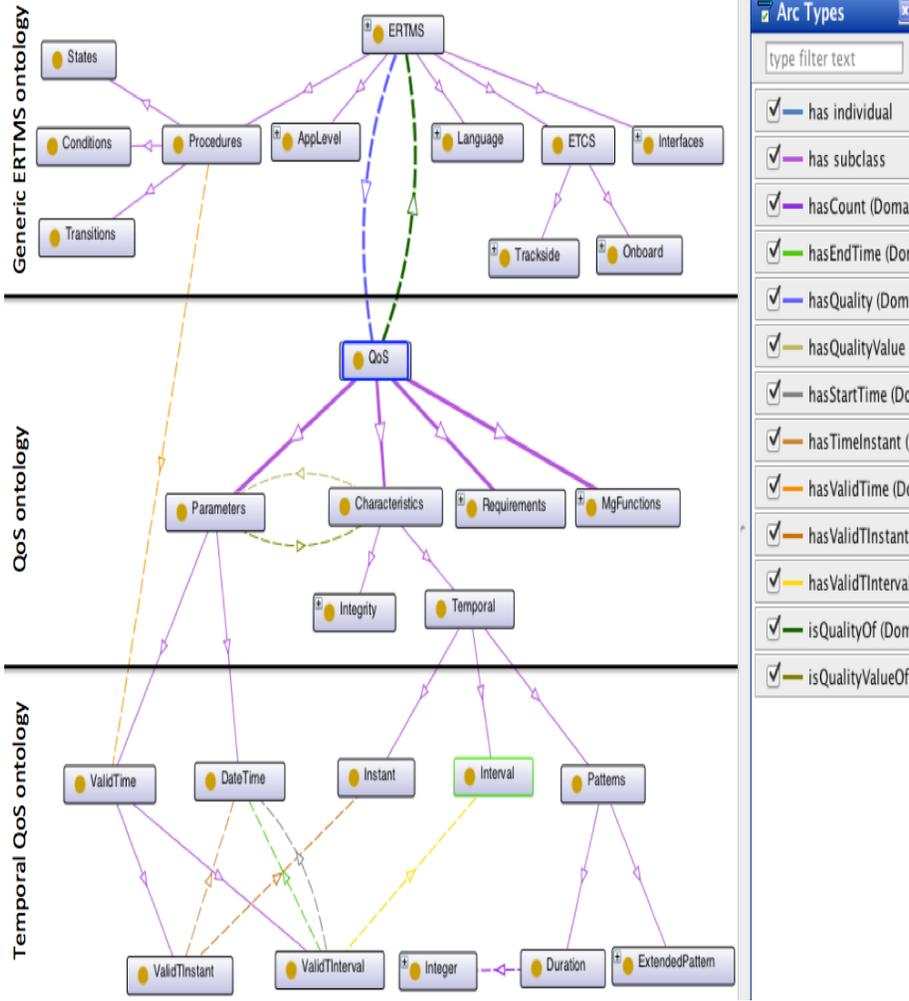
Fig. 4 3-Layer Temporal QoS Ontology for ERTMS/ETCS
