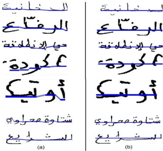
Fig. 3. (a) Extracted baseline, (b) baseline by horizontal projection
