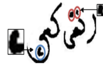
Fig. 5. Diacritic points extraction from the word التركي.
