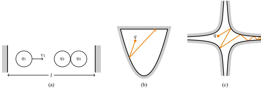
Fig. 1. Examples of systems with unilateral constraints. (a) 3-ball chain with walls. (b) Nonlinear billiard. (c) Non-convex billiard.
