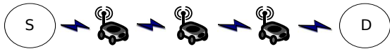
Fig. 4. Multiple routers scenario composed of three mobile routers, one source node, and one destination node.
