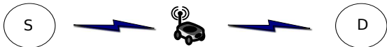
Fig. 2. Basic scenario composed of one mobile router, one source node, and one destination node.
