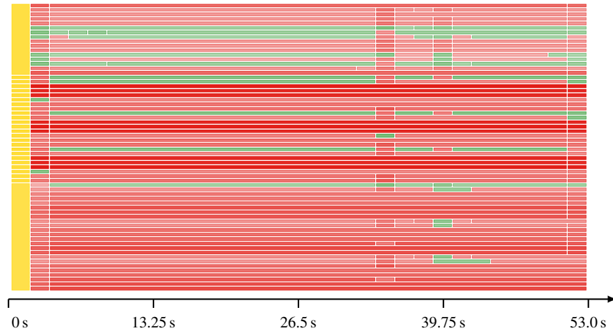
Fig. 5 Spatiotemporal overview of the application shown by Figure 3. We still see the two temporal perturbations (around 35 and 40 s). State colors correspond to following the MPI calls: Yellow - MPI_Init, Green - MPI_Send, Red - MPI_Wait
