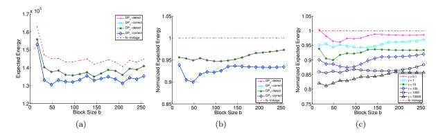
Figure 2: Impact of b and  $\gamma$  on the expected energy consumption for zero voltage switching cost. Only the results for the  $DP_n$ -correct algorithm are shown in (c).
