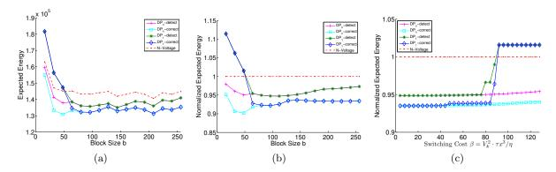
Figure 4: Impact of b and  $\beta$  on the expected energy consumption. In (a) and (b), the voltage switching cost is equivalent to the energy consumed to multiply two  $32 \times 32$  matrices at nominal voltage without overhead, i.e.,  $\beta = V_k^2 \cdot \tau \cdot 32^3/\eta$ .
