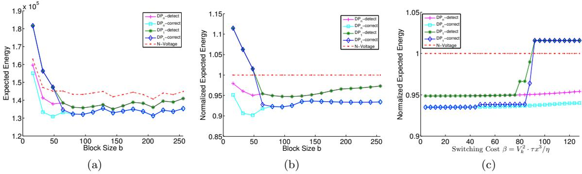
Figure 4: Impact of  $b$  and  $\beta$  on the expected energy consumption. In (a) and (b), the voltage switching cost is equivalent to the energy consumed to multiply two  $32 \times 32$  matrices at nominal voltage without overhead, i.e.,  $\beta = V_k^2 \cdot \tau \cdot 32^3 / \eta$ .
