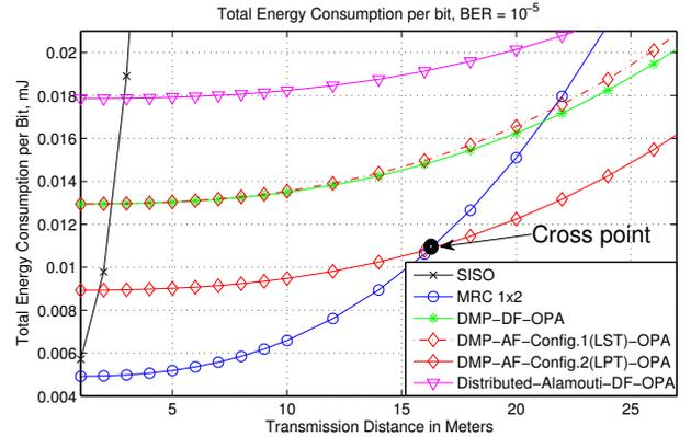
Fig. 4. Total energy consumption vs. distance ( $10^{-5}$  BER)
