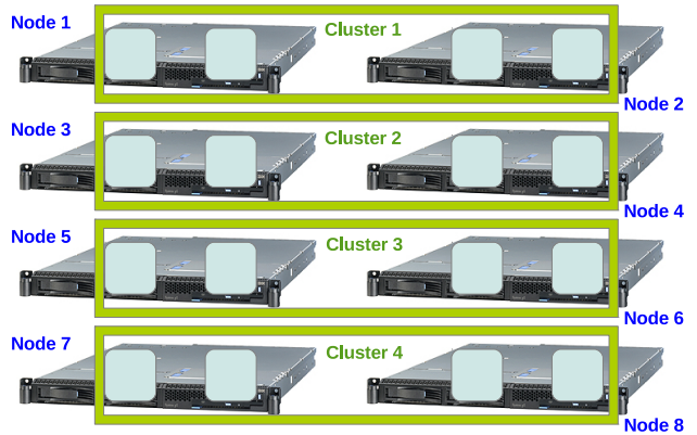
Fig. 2. Failure containment protocol clustering
