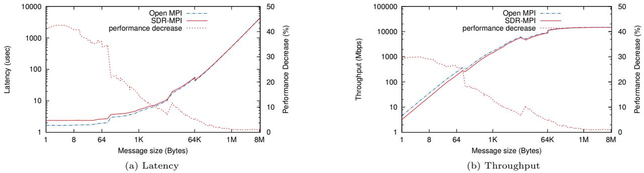
Figure 7: Performance of SDR-MPI on InfiniBand-20G (replication degree=2)
