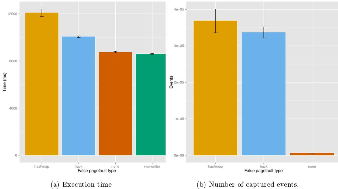
Figure 3: Impact of the false page faults mechanism on a parallel matrix multiplication of  $1000^2$  doubles.
