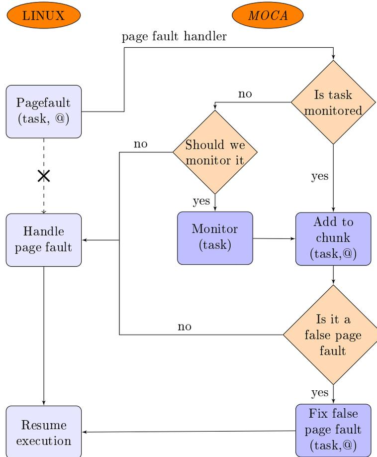
Figure 1: Flow chart of *MOCA*'s page faults
