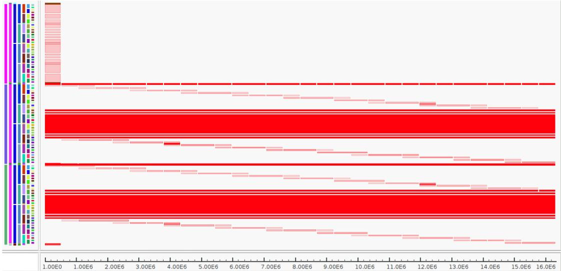
Figure 4: Memory-gantt view of a parallel matrix multiplication.
