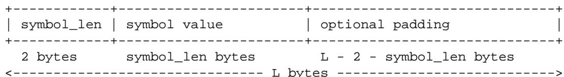
Figure 1: Symbol Format, Case of a Single Flow
