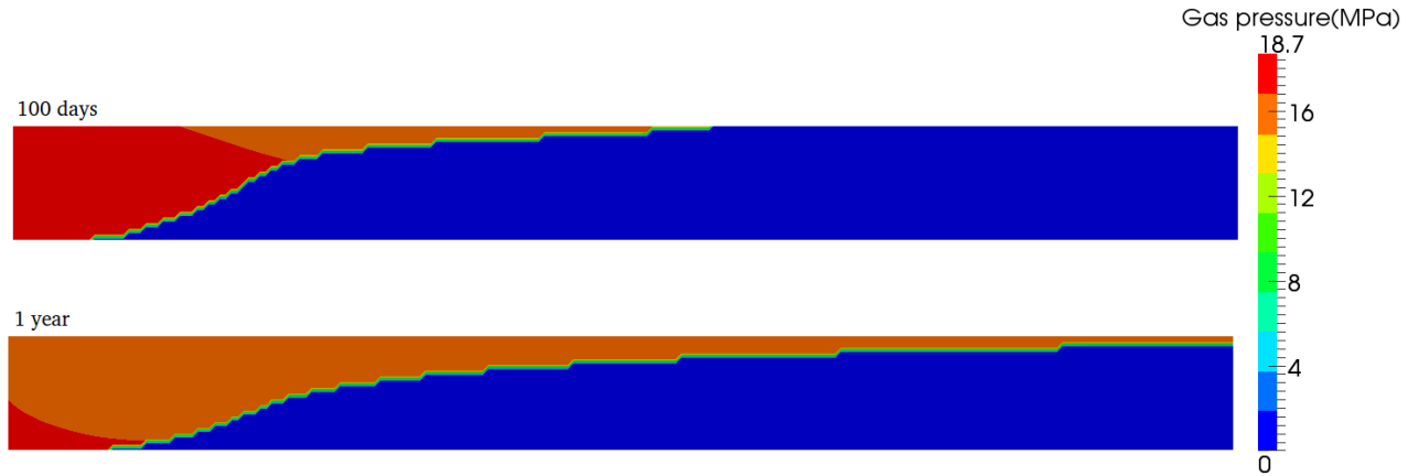
FIGURE 4. Gas pressure P_g after 100 days and 1 year of CO 2 injection. Only the 1.1 km closest to the injection is presented.
