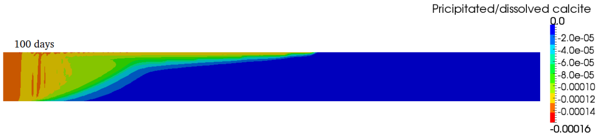
FIGURE 6. Precipitated/dissolved calcite volume fraction after 100 days of \text{CO}_2 injection. Only the 1.1 km closest to the injection is presented.
