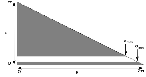
Figure 3: Constraining the projection of targets A and B in on-screen convex shapes s_A and s_B reduces the domain of variable \alpha in the Toric space. The set of cameras which satisfy the framing constraint (white area) is then given by a horizontal strip \alpha \in [\alpha_{\min}, \alpha_{\max}] in the plane (\theta, \alpha) .
