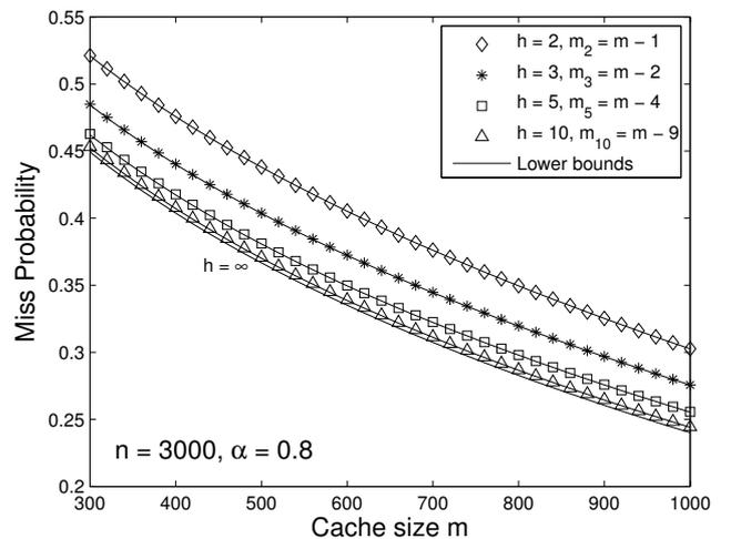
**Figure 1: Lower bounds for  $h = 2, 3, 5, 10$  and  $\infty$  and the miss rate  $M(\mathbf{m})$  with  $m_1 = \dots = m_{h-1} = 1$  for  $h = 2, 3, 5$  and  $10$  as a function of the cache size  $m$ , with  $n = 3000$  and  $\alpha = 0.8$ .**
