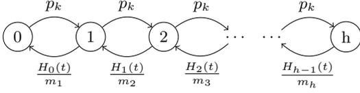
**Figure 2: Evolution of the list in which item  $k$  is. When  $p_k$  is small and the  $m_i$ s are large, the state of one item becomes independent of the hit rate in each box and its behavior can be approximated by a time-inhomogeneous continuous-time Markov chain. This is the mean-field approximation.**
