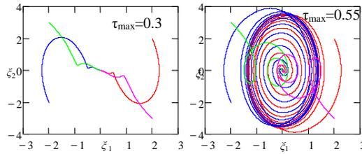
Figure 1. Trajectories of stabilized delayed double integrator
