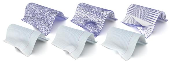
Figure 5: Comparison with other methods. *The Standard FEM (left) and Narain *et al.* [10] method (middle) required a very dense mesh in order to get a result of similar visual quality as our method (right).*
