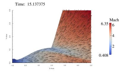
Figure 24: Mach number and velocity vectors at steady state for  $P_c/P_{atm}=2000$ .
