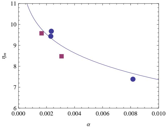
FIG. 2: Universal plot  $\eta_m$  vs  $\alpha = N(\hbar\bar{\omega}/k_B T)^3(1 - e^{-4\eta_*})$  (blue curve). The blue solid circles correspond to the results obtained for  $^{133}\text{Cs}$  in Fig. 3(a) with  $\eta_* = 0.098$ . The red solid squares correspond to the  $^7\text{Li}$  data of Fig. 3(c) with  $\eta_* = 0.21$ .
