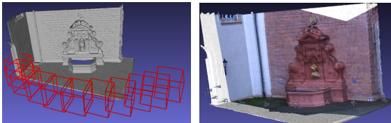
Figure 5: Fountain: (left) 11 cameras 2m Bbx and scene, (right) estimated cameras in textured scene using SSR.
