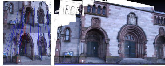
Figure 6: Herz-Jesu: (left) matched 2D features with outliers in red, (right) texture-mapped scene using RR.
