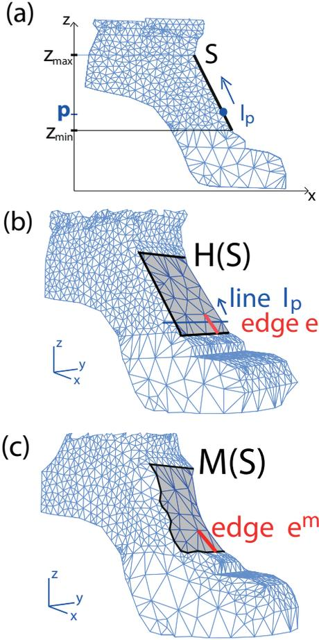
Fig. 7. Protruding edges composing the silhouette: (a) Silhouette with selected silhouette line  $S$  and marching parameter  $p$ . (b) Silhouette hull triangulation  $H(S)$  with marching line  $l_p$ . As the marching line advances, we select the most protruding edge among those intersecting  $l_p$ . (c) Current mesh  $M$  with selected edge in red.
