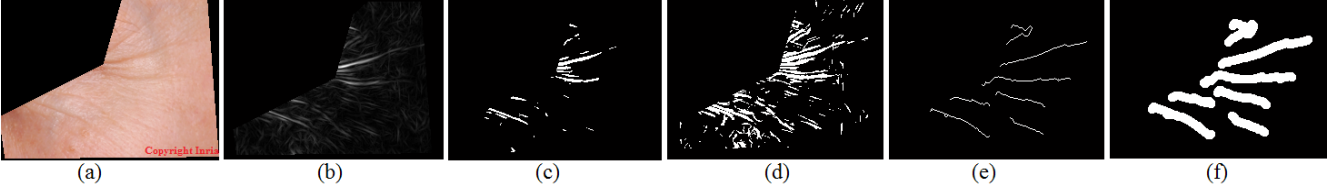
Fig. 3. Formation of image template. (a) Input image. (b) Gabor features. (c) Gabor features with a higher threshold value. (d) Gabor features with a lower threshold value. (e) Output of wrinkle detection algorithm. (f) Detected wrinkles dilated with a circular disc.
