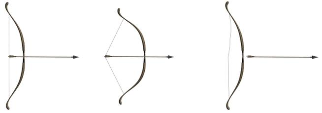
**Figure 7:** A bow physically shooting an arrow. (Left) At rest, an inextensible string slightly bends a stiff solid wood frame. (Middle) Applying a force on the string significantly bends the frame. (Right) When released, the string is tightened by the wood which comes back to its rest position, projects the arrow then oscillates.
