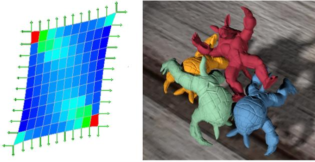
**Figure 6:** Complex materials. Left: A patch of anisotropic quads pulled by external forces (Von Mises Stress texturing). Right: Four armadillos, all simulated by different materials (red rigid body, green plastic tetra FEM, blue Neo-Hookean hexa FEM, yellow St Venant-Kirchhoff meshless), are colliding using unilateral constraints.
