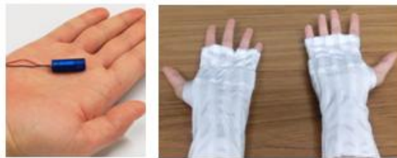
Fig. 4. Left: A vibration motor. Right: Our gloves with 10 embedded motors (5 per hand). In the tactile feedback condition, individual motors are activated to represent the classifier output.
