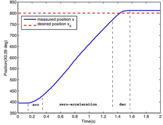
Fig. 5. A trajectory with SSE under built-in controller
