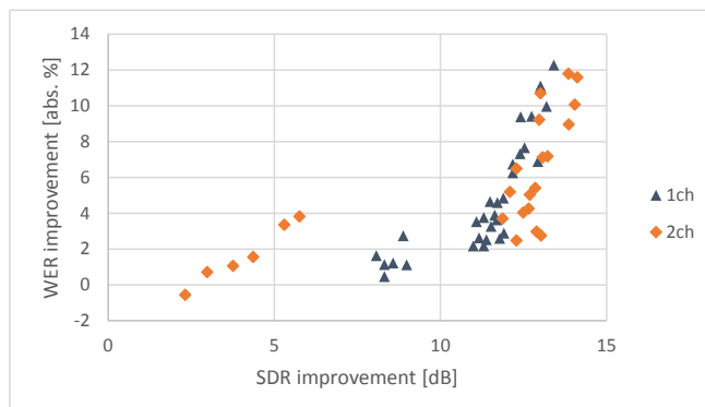
Fig. 1. Relation between improvements in source separation performance (SDR) and word error rate (WER).
