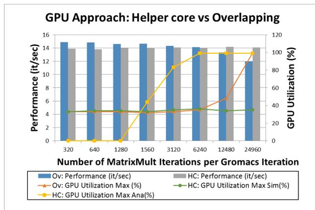
**Fig. 4.** Helper core (HC) and overlapping (Ov) strategies when increasing the number  $y$  of matrix multiplications perform per Gromacs Iteration. The GPU utilization for helper core strategy is split in two curves. GPU Utilization Max Sim indicates the maximum utilization of the 7 GPUs used by the simulation. GPU Utilization Max Ana is the GPU utilization for the GPU used by the in situ multMatrix.
