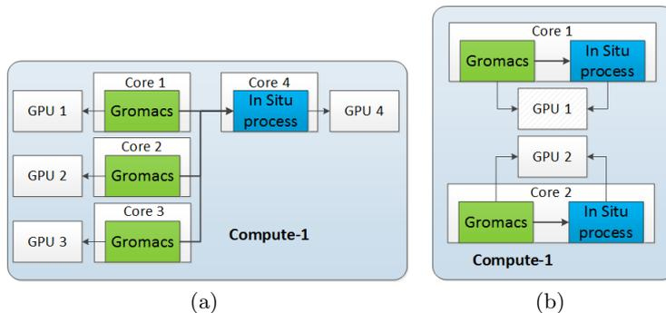
**Fig. 1.** (a) Helper core strategy. A dedicated core is allocated for in situ analytics. Data are gathered by the node and sent asynchronously to the in situ tasks (b) overlapping strategy. One in situ task is instantiated for each MPI process of the simulation.
