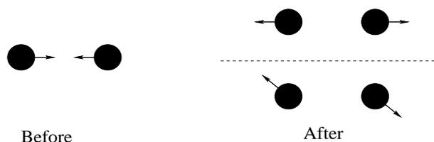
**Fig. 2:** The figure demonstrates how the outcome of a collision in two or more dimensions is not uniquely defined by conservation of energy and momentum. Both of the two final states on the right are consistent with the conservation laws.
