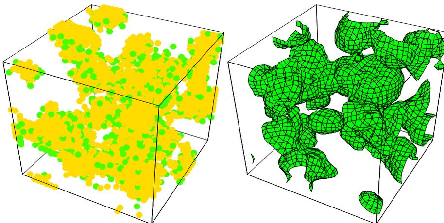
**Fig. 3:** Bi-continuous (worm-like) phase of amphiphilic pentamers. To the left we show the individual molecules explicitly (except for water which is not shown). Hydrophilic head groups are shown in green while the hydrophobic tail monomers are shown in yellow. The figure on the right shows iso-density contours of the amphiphilic polymers.
