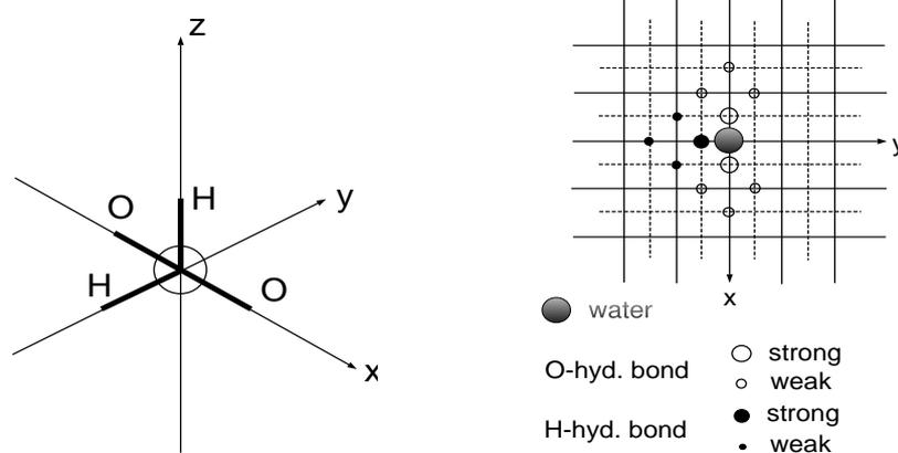
**Fig. 1:** The figure on the left shows the geometrical structure of the water molecules. The right figure shows a two dimensional slice of the local field configuration building up the hydrogen bonds.
