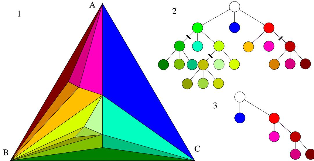
**Fig. 2:** A random Apollonian network structure of order 7 (1), its corresponding tree  $T$  (with the neighborhood of the center delimited by cuts on the branches) (2) and the  $\bar{T}$ -subtree of  $T$  (3).
