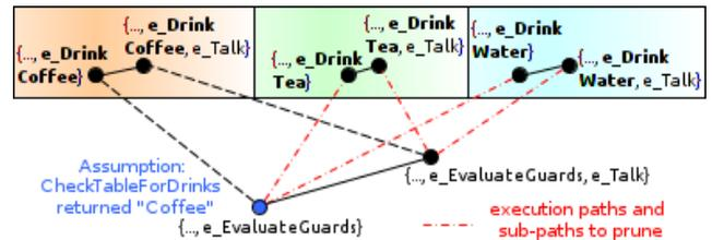
**Figure 6.** Close-up on the simplified Event Structure of the example model where the Feedback Protocol is applied. Dashed lines represent data-dependent causalities. Red dots-and-dashes lines represent the execution paths that must be pruned as a result of the Feedback Protocol if the “CheckTableForDrinks” node returned “Coffee”.
