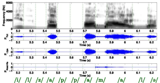
**Figure 4:** a) Wide-band spectrogram of the simulated utterance /ilzap'amalə/, b) total acoustic pressure signal, c) acoustic pressure radiated at the lips, and d) acoustic pressure radiated at the nostrils. Phonetic segmentation is indicated by dashed line.
