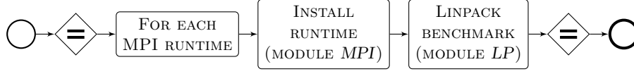
Fig. 1. High-level workflow description of the exemplary experiment (modified BPMN notation). Each runtime is sequentially installed and evaluated with Linpack benchmark. Note that some parts of the workflow refer to external repositories.
