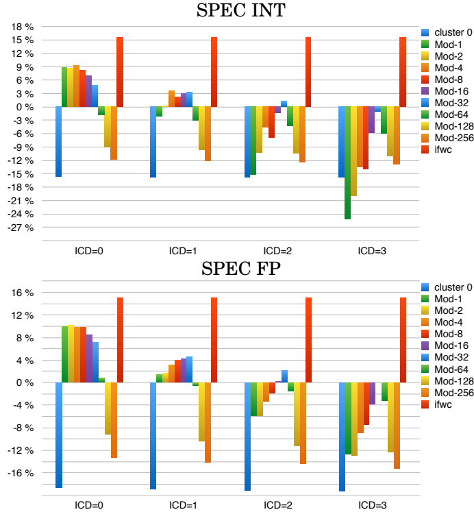
Fig. 5. IPC gain over the baseline for clustered iiffccw configurations, for inter-cluster delays (ICD) of 0,1,2 and 3 cycles, under a Mod-N steering policy with N ranging from 1 to 256. The leftmost bar of each group of bars is the IPC gain when steering all the micro-ops to cluster 0. The rightmost bar is the IPC gain of the non-clustered ifwc configuration. The top graph is the average for SPEC INT, the bottom one for SPEC FP.
