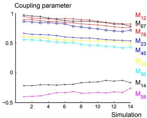
Fig. 6: The extracted inter-resonator couplings for each simulation.
