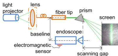
Figure 1. System setup of the endoscope and optical fiber.
