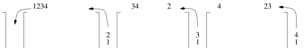
Fig. 1: Four steps in the sequence of operations that outputs 2341 from 1234 using a single stack. Each arrow shows an operation that is about to be performed.
