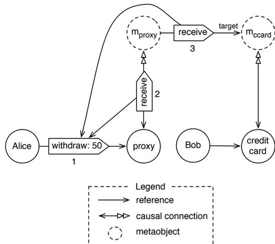
**Figure 2.** Bob has created a proxy for its credit card and passed it to Alice. When Alice sends a message to the proxy (1), the proxy sends a receive message to its metaobject with a reification of Alice message (2). The metaobject of the proxy can then decide whether to forward the message to the metaobject of the credit card (3). Bob can still use his credit card directly.
