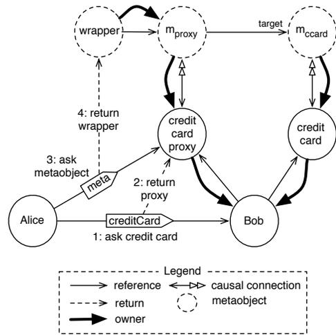
**Figure 3.** Proxy protection: (1) Alice asks Bob for his credit card, (2) Bob creates a proxy for his credit card to limit withdrawals and returns it, (3) Alice asks for the metaobject of the proxy to leak the credit card (target of the proxy), (4) but Alice does not own the proxy: she obtains a wrapper on the metaobject of the proxy and cannot leak the credit card.
