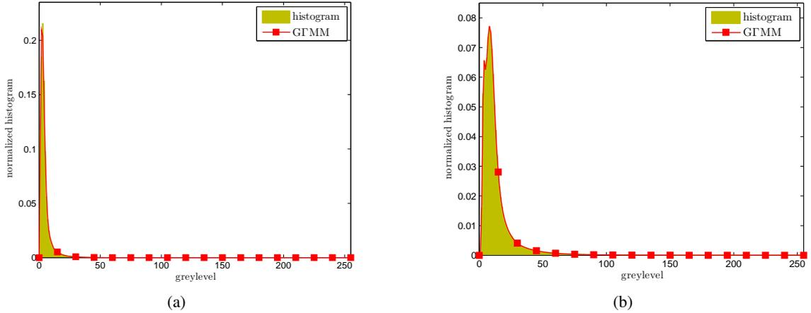
Fig. 9. Histogram and the estimated PDFs of HECM-FJ-GMFM on the “Port-au-Prince16” COSMO-SkyMed image: (a) 8-bit uniformly-compressed version, and (b) 8-bit compressed statistics after truncation.
