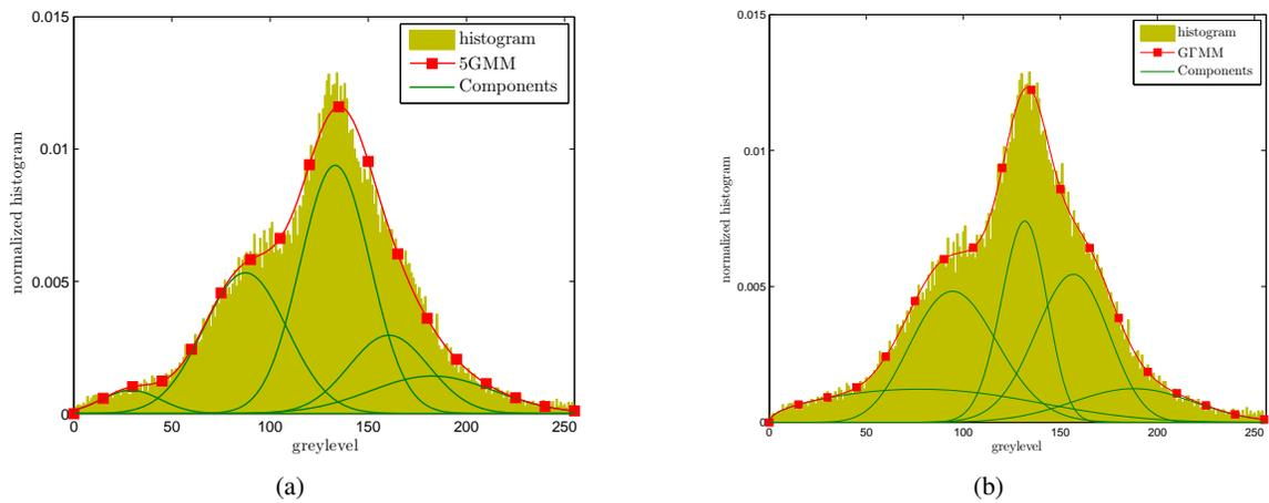
Fig. 12. Histogram and the estimated PDF of 5GMM and GM with the plots of components for the “Toulouse” image: (a) 5GMM, and (b) GM.
