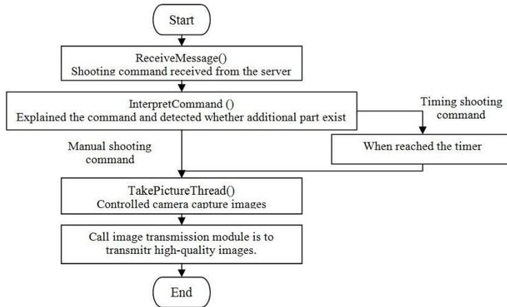
Fig. 4. The process of the shooting module
