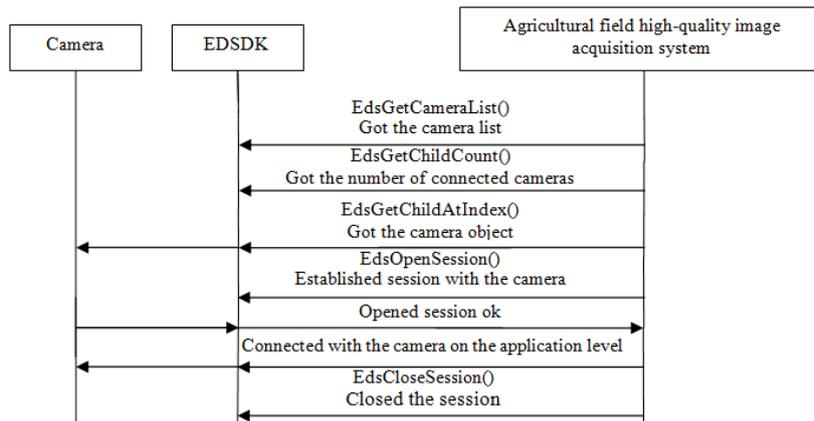
Fig. 3. The process of accessing the camera
