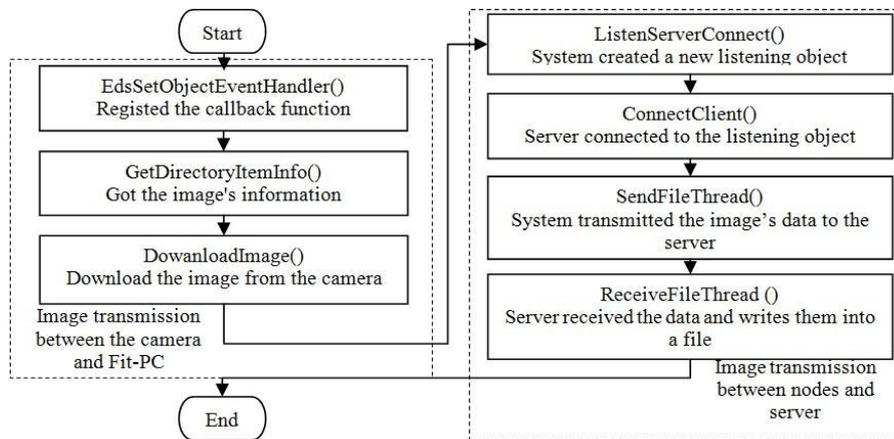
**Fig. 5.** The process of image transmission module
