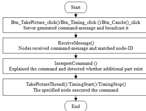
**Fig. 6.** The process of the command response module
