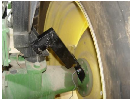
Fig.4. Setting of speed sensor
