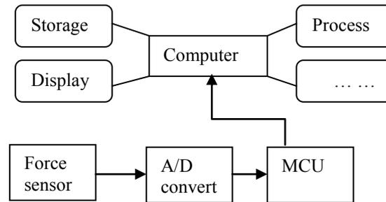
**Fig. 2.** Frame diagram of data acquisition and processing
