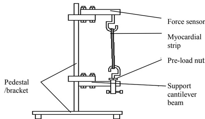
Fig. 1. Schematic of contractile force detecting device
