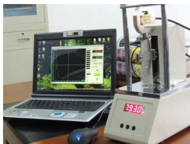
Fig. 1. Test equipment and test process of shear modulus
