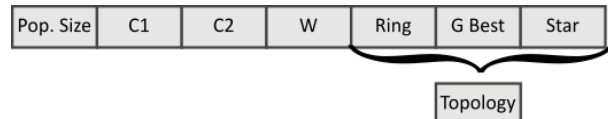
Figure 1: Representation of a set of PSO parameters inside the tuner. The first four elements represent numerical parameters (either integer or real-valued numbers), while the last three contribute to the decision about a nominal parameter (in this case topology).
