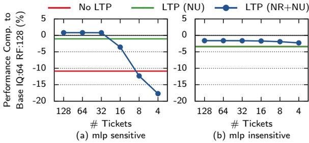
**Figure 11: Performance impact of varying number of tickets for an LTP design with both *Non-Urgent* and *Non-Ready*.** The red line shows the results for IQ 32/RF 96 without LTP, and the green line shows the results of NU-only with a 128-entry LTP with 4 ports.
