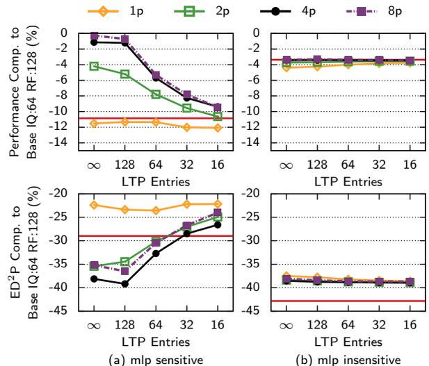
**Figure 10: Performance and Energy (IQ/RF) impact of varying LTP size and number of ports for an LTP/IQ 32/RF 96 design relative to the IQ 64/RF 128 baseline. The redline shows the results for IQ 32/RF 96 without LTP.**
