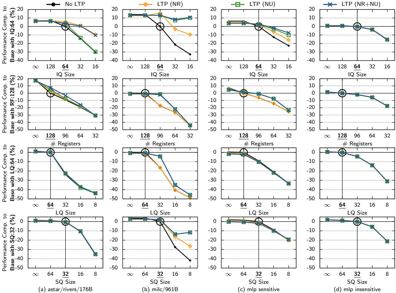
**Figure 6: Limit study: Impact of IQ, RF, LQ, and SQ resource sizes with and without LTP. The baseline configuration for each resource is underlined on the x-axis and indicated with a circle. (Prefetcher enabled, unlimited MSHRs.)**
