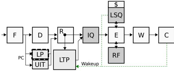
**Figure 8: LTP Overview.** The Urgent Instruction Table (UIT) (and Long-latency Predictor (LP) for Non-Ready instructions) are accessed early in the pipeline to decide whether instructions should be parked in LTP at the rename stage. Wakeup signals come from completing instructions later in the pipeline.
