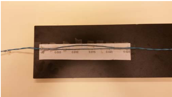
Fig. 1: Untwisted pair with a cosine profile D(z) .
