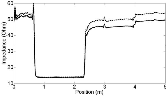
Fig. 4 Comparison of two  $Z_0(z)$  profiles obtained by inverse scattering on the same line including an (equivalent) segment of  $25 \Omega$  with zero padding up to  $15 \text{ GHz}$  (-) and  $30 \text{ GHz}$  (- -). These results show that a higher zero padding leads to a more accurate result
