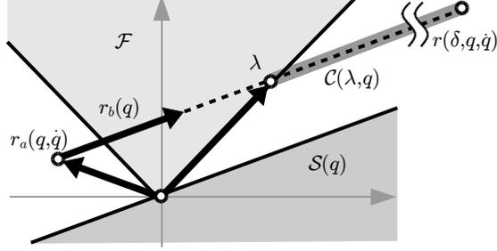
**Fig. 6** Geometric interpretation of (114) of the case of  $G_A(q, \dot{q}) > 0$  and  $G_B(q) > 0$ , where the unique solution  $\lambda$  exists.
