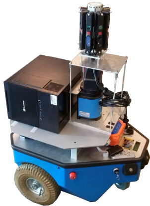
Figure 11: Robot with the omnidirectional RGB-D sensor.
